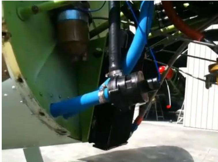
Figure 6.5: Installation of a 15 L/min booster pump
