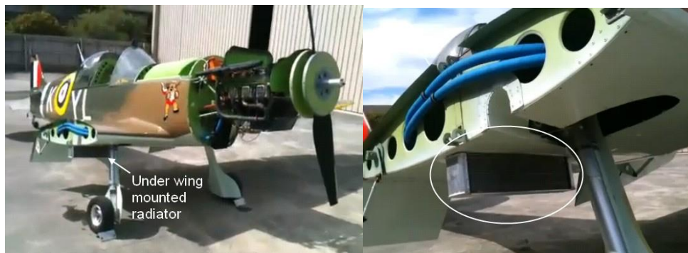
Figure 6.4: Radiator mounted under wing.
